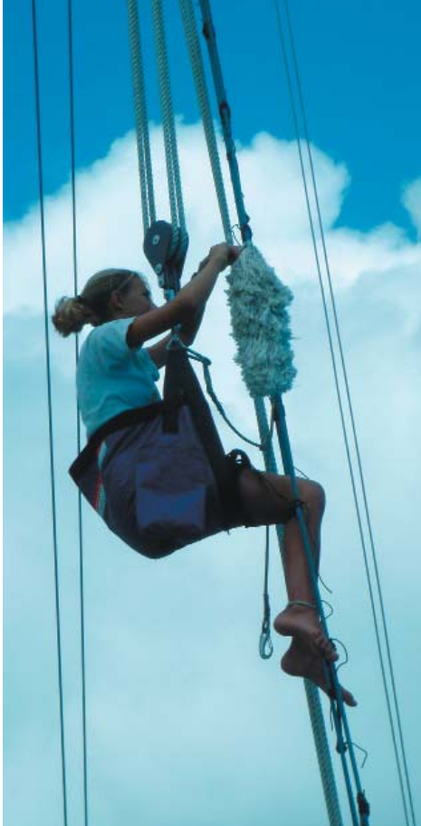
Alexis Bach installing baggywrinkles
